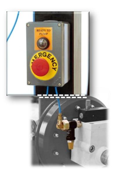
Emergency on-off control to stop the pump by a start-stop pushbutton
